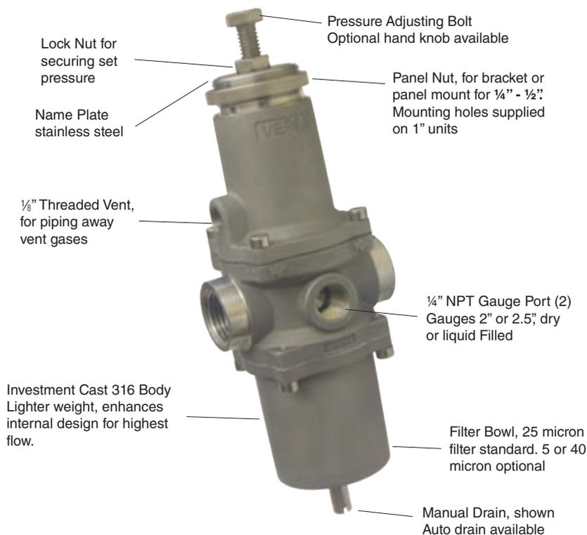
The Versa Type AR-316 series of stainless steel regulators and filter regulators are designed to stand up to the harshest environments while providing highly accurate pressure regulation.
